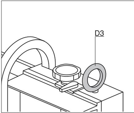
b) If using a crane, the crane hooks **(D3)** should be used to lift the machine.
