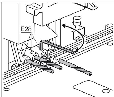
Use a hex wrench to loosen the grub screw (E28)
