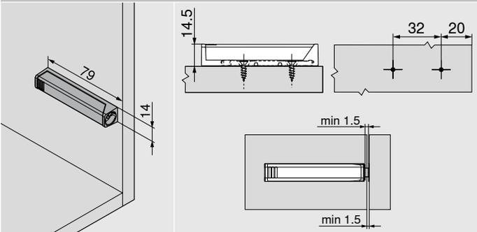
Technical drawing showing the installation of the long support. It includes a perspective view with dimensions 79 mm length and 14 mm height. A cross-section shows a 14.5 mm depth. A top view shows two mounting holes with a 32 mm spacing and a 20 mm total width. A side view shows a minimum 1.5 mm overlap on both ends.
