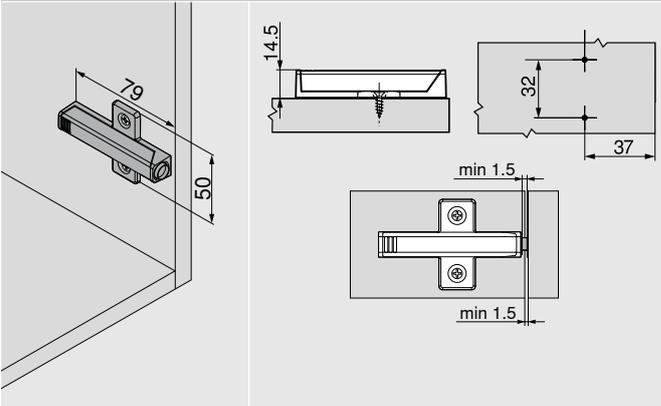
Technical drawing showing the installation of the long support with a crossbar. It includes a perspective view with dimensions 79 mm length, 50 mm height, and 14.5 mm depth. A top view shows two mounting holes with a 32 mm spacing and a 37 mm total width. A side view shows a minimum 1.5 mm overlap on both ends.
