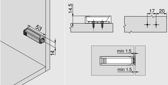
Technical drawing showing the installation of the short support. It includes a perspective view with dimensions 53 mm length and 14 mm height. A cross-section shows a 14.5 mm depth. A top view shows two mounting holes with a 17 mm spacing and a 20 mm total width. A side view shows a minimum 1.5 mm overlap on both ends.
