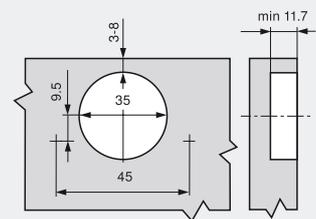
\* Dimension for mounting plate with dimension A = 37 mm
