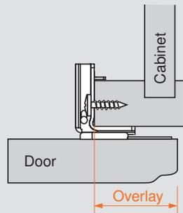
Cabinet overlay refers to the amount the cabinet door overlaps the cabinet opening. The overlay dimension is how much bigger the door is than the cabinet frame.
