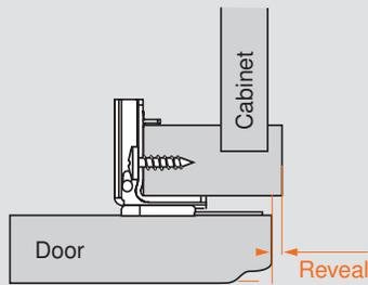
A reveal is the portion of the cabinet frame left exposed after the door is attached. Even with full overlay applications, a reveal is needed
