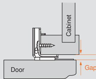
The gap is the distance between the cabinet door and the cabinet when looking at the side of the cabinet. The gap prevents the doors from binding.
