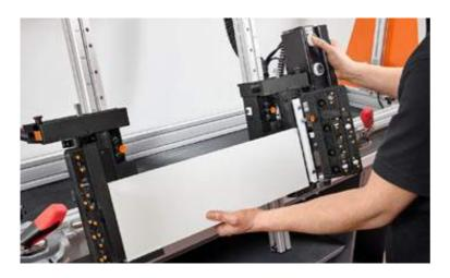
Assemble different back heights and widths. Thanks to pneumatic clamping, you no longer need to set stops.
