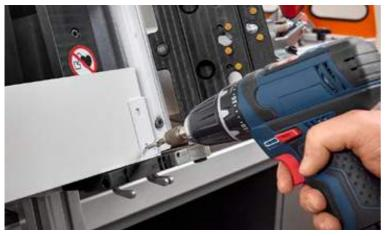
Nail or screw the back fixing to the chipboard back.
