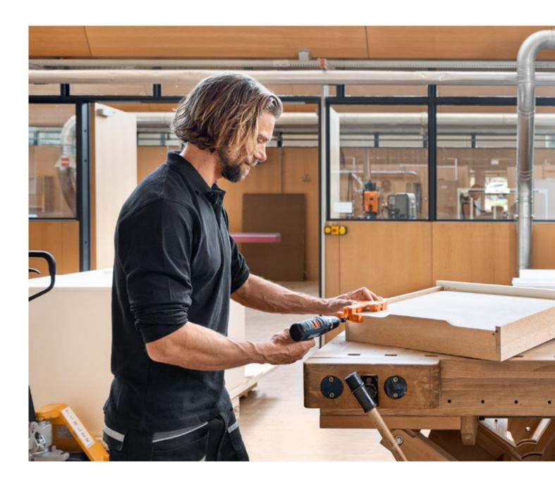
Pre-drilling allows fittings to be set even more precisely. This is particularly useful for wood and therefore also for fixing the runner profile to the drawer. You can determine the exact drilling position particularly efficiently using our drilling templates. And your work will be even easier with MINIPRESS top. If your drawers are correctly positioned on the runner profile, their feather-light glide is guaranteed.
