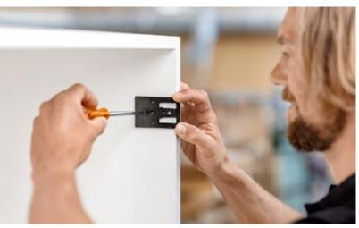
Our assembly devices assist you in processes such as positioning and fastening the AVENTOS lift mechanism to the cabinet. Optimal alignment ensures that the fittings function perfectly, making opening and closing a pleasant experience for your customers.
