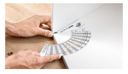
When it comes to mounting the fronts, we have further assembly devices in our range. These include our drilling templates for hinges, which ensure that the drilling positions on the front match those on the cabinet precisely. This results in hinges working perfectly – the doors close beautifully and the gap layout is faultless.
