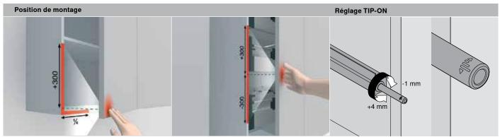
Optimal opening support is ensured when the TIP-ON unit is attached in the correct handle position.
