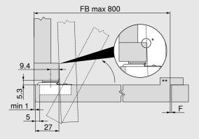
Hinge dimensions and gap calculation based on factory setting \* prevent collision
